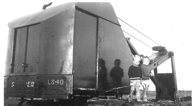
A Tom Johnson designed (to dump forward) land-clearing shovel about 1938 (Paul and Don in front)
